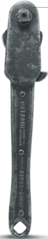
MATADOR's first reversible ratchet made in 1924, patented in Germany.
